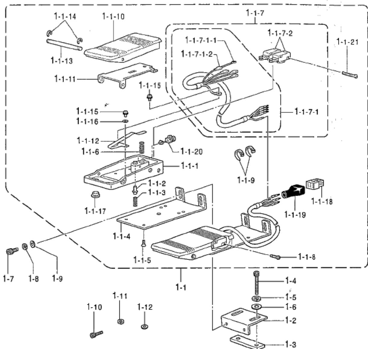
V1. 踏板関係 / Foot switch pedal mechanism
