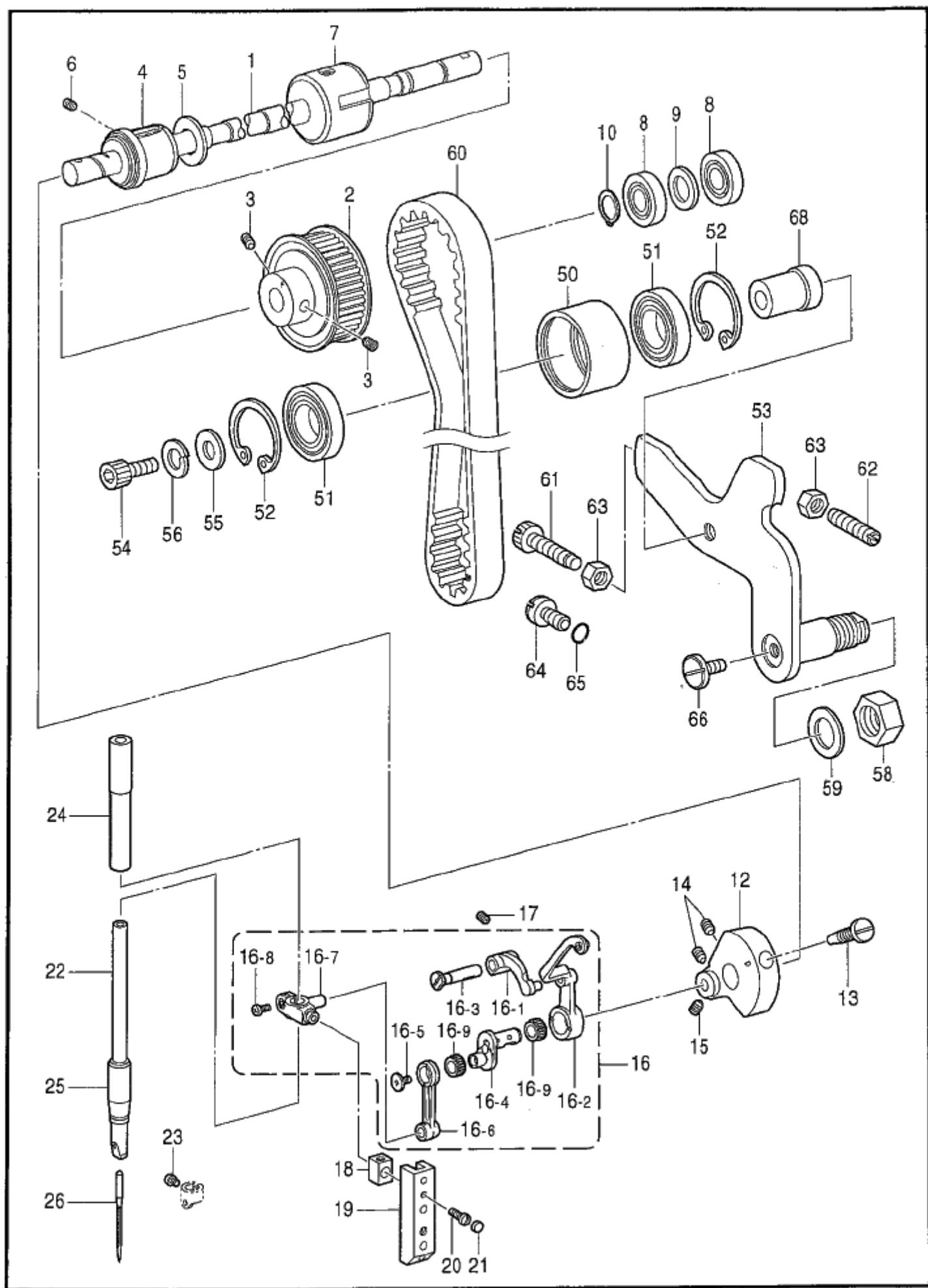
B1. 上軸・針棒関係 / Upper shaft and needle bar mechanism
