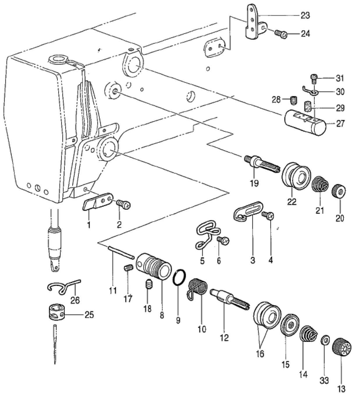
H. 糸通し関係 / Threading mechanism
