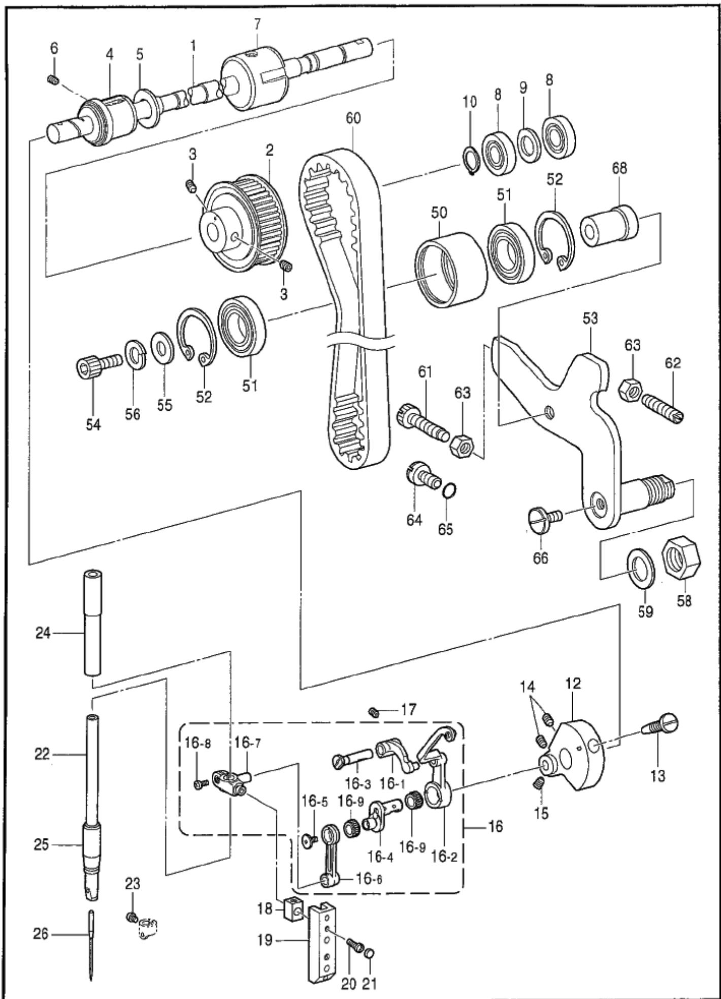
B1. 上軸・針棒関係 / Upper shaft and needle bar mechanism
